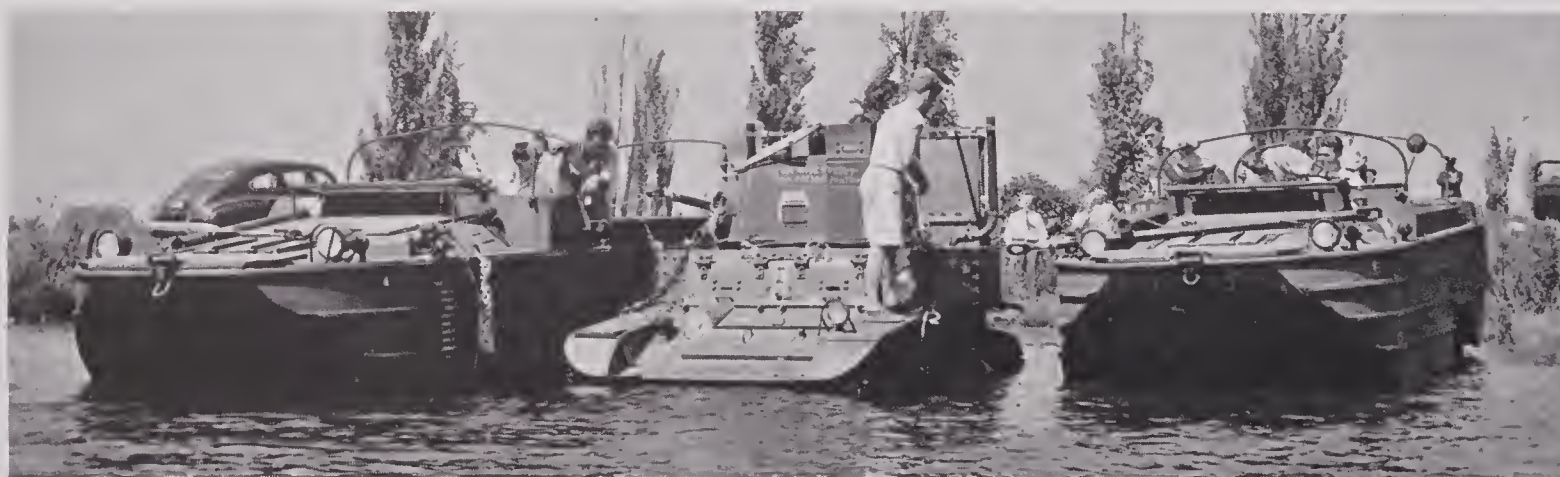
FIGURE 60. Light tank being connected to two DUKWs for wet ferry across Sloan Lake at General Motors Corporation Proving Grounds, Milford, Michigan.
